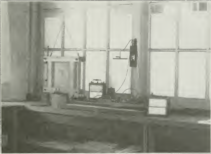
General arrangement of apparatus, showing the ammeter, voltmeter, wheatstone bridge, and reflecting galvanometer.
